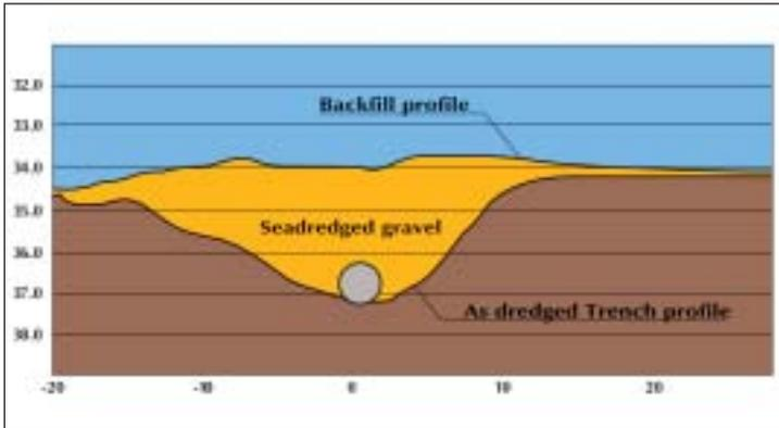
Figure 4. A trench profile in the Westhinder Shipping Channel before and after backfilling.
