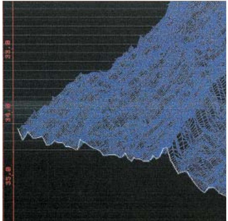
Figure 3. The on-line multibeam survey which was installed on the dredger *Cristoforo Colombo* shows the position of the Zeepipe installation.
