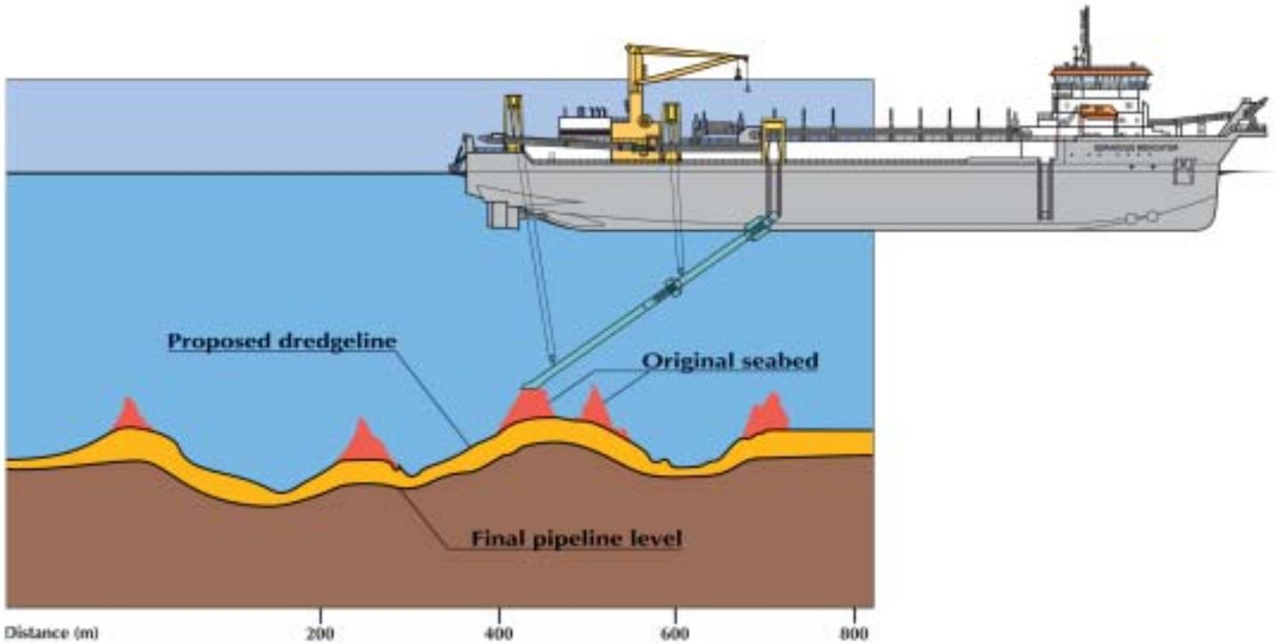
Figure 2. A typical presweep longitudinal profile.
