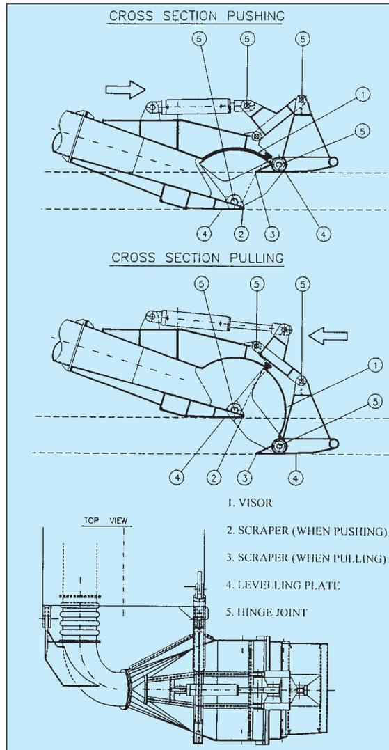
Figure 3. The sweep-head (general lay-out).
