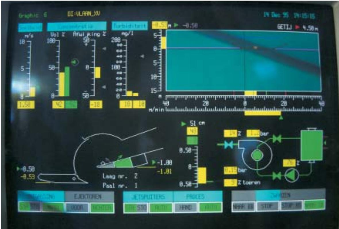
Figure 6 : Computer controlled dredging operations.
