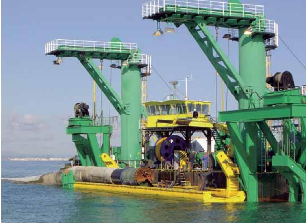
Figure 15. Pipe coupling pontoon Manta.
