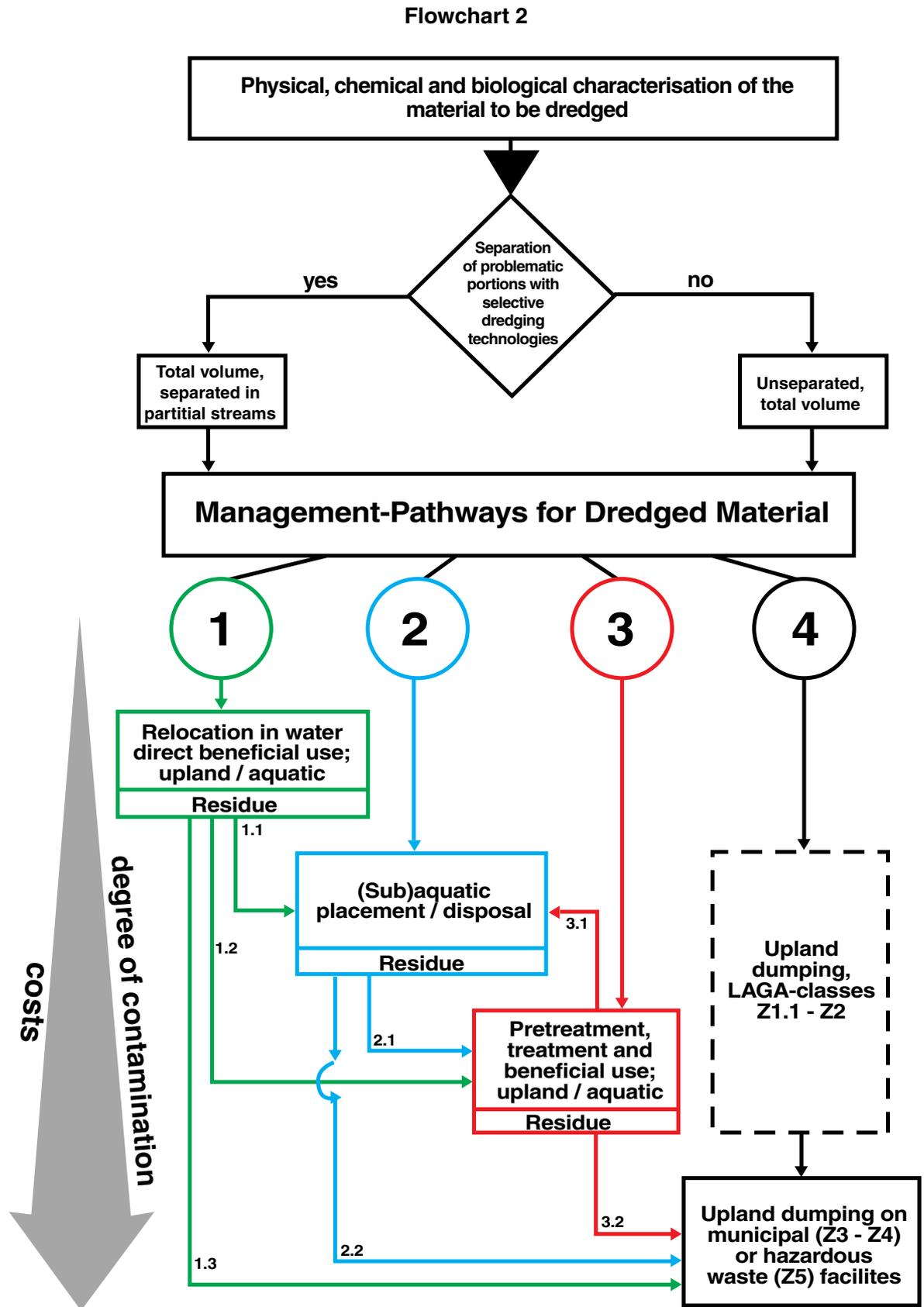
Figure 6. Basic possibilities for the management of dredged material.
