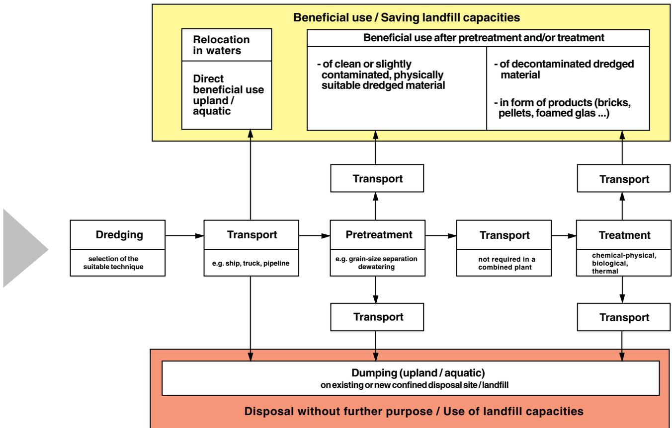
Figure 5. Management scheme for dredged material: Cost-relevant handling steps of the partial streams.
