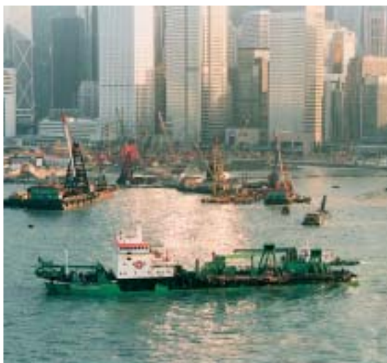
Figure 6. The splithull trailer dredger Krankeloon proved environmentally acceptable for the work.
