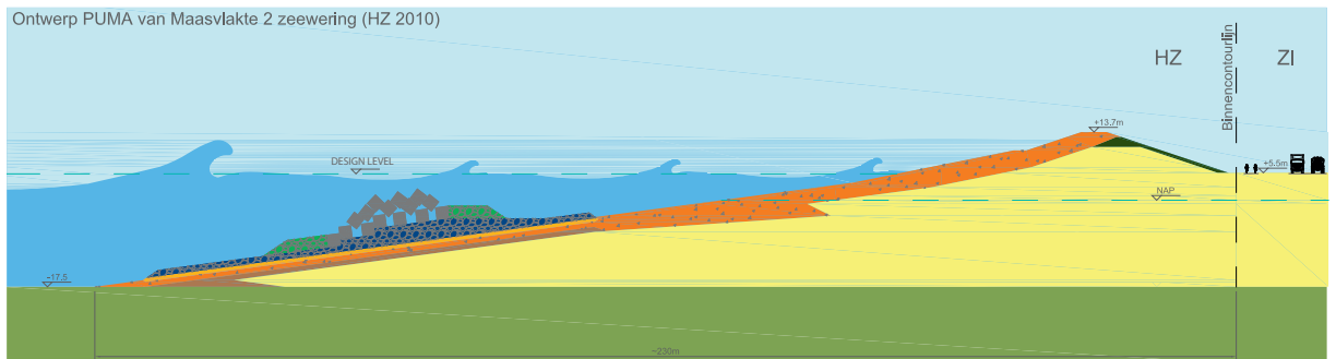
Figure 8. Partnering result: cobble beach and dune with concrete cube reef, length 3.5 km.
