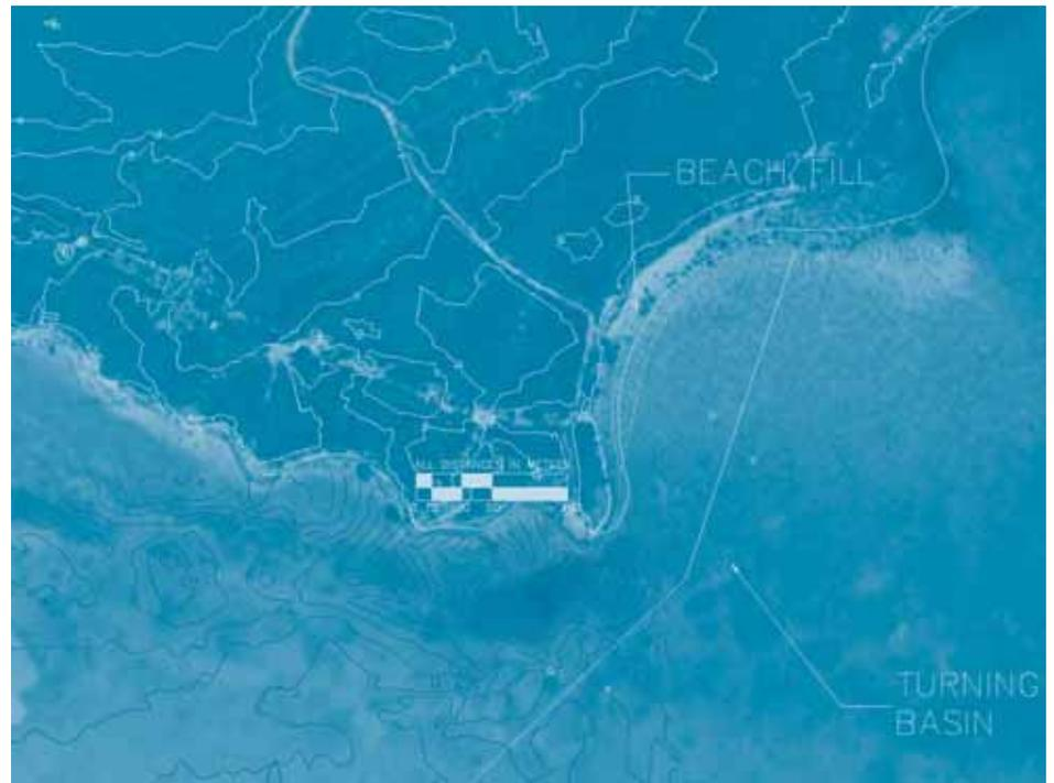
Figure 15. Water Cay beach fill, turning basin, and containment area.
