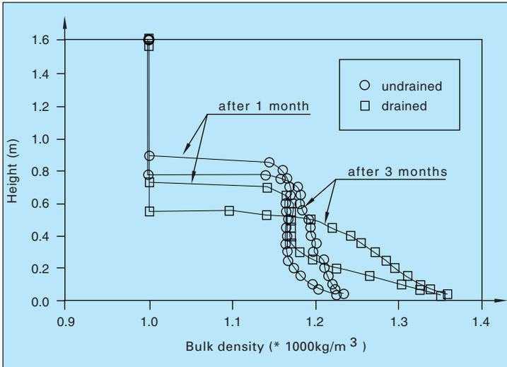
Figure 7. Density profiles for columns KO5 (undrained) and KO6 (drained).
