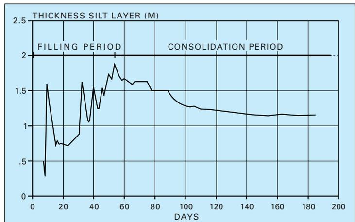
Figure 2. Layer thickness in a dewatering field.
