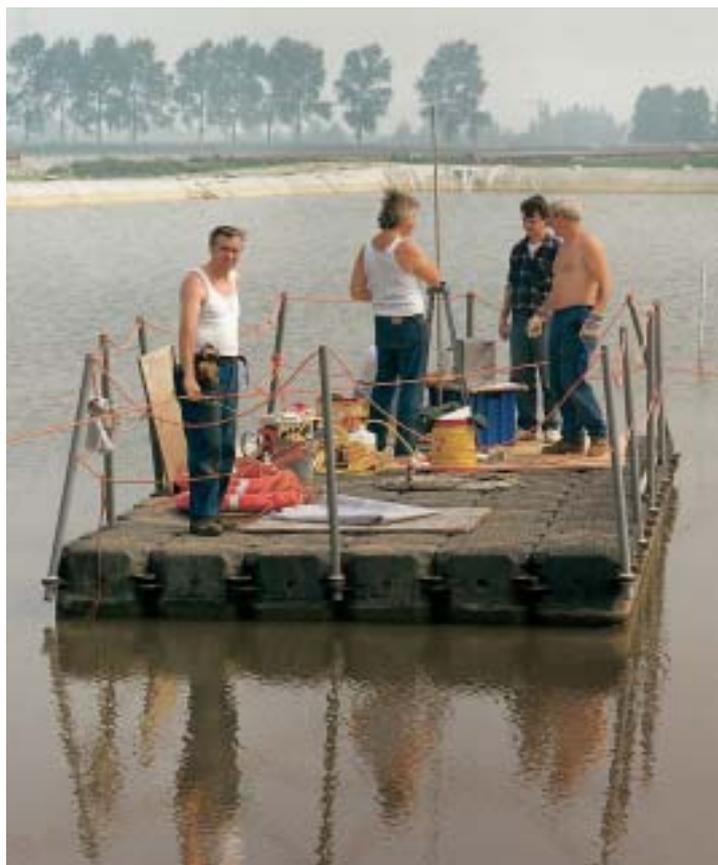
Figure 9. In-situ sampling and density measurement pontoon.
