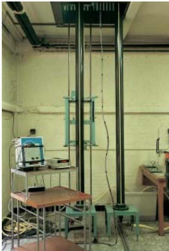
Figure 6. Consolidation column set-up in laboratory.
