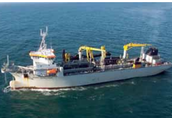
Figure 11. The trailing hopper dredger Filippo Brunelleschi was used for seabed levelling at 70 m water depth.
