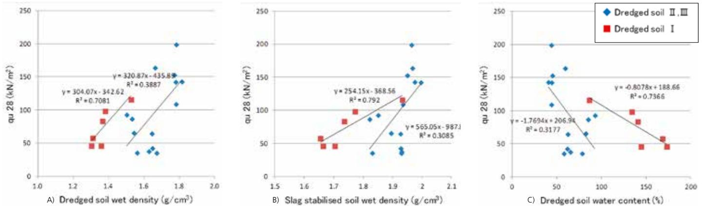
Figure 11. A) Relationship between wet water density of dredged soil and qu28; B) between wet water density of converter slag and qu28; and C) between content ration of dredged soil and qu28.
