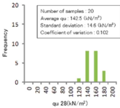
Figure 13. Strength distribution of qu28 (dredged soil I).
