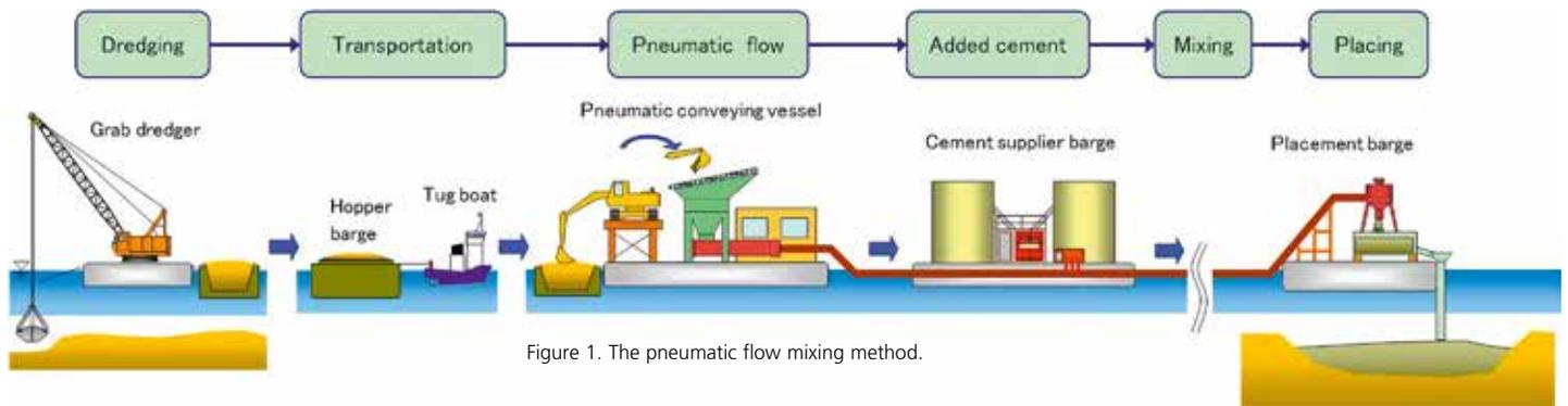
Figure 1. The pneumatic flow mixing method.
