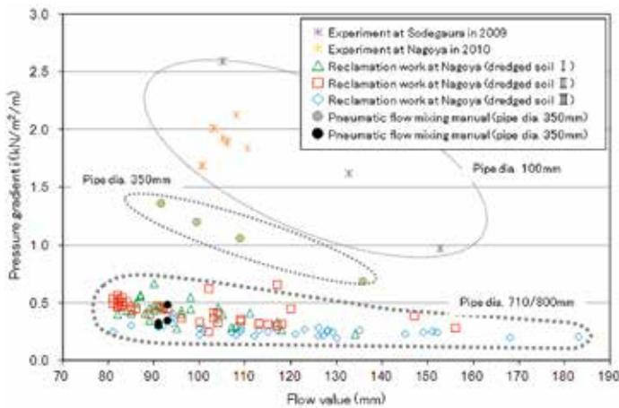
Figure 17. Relationship between flow value of slag stabilised soil and pressure incline.
