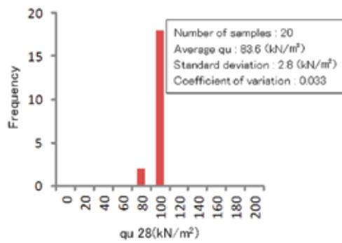
Figure 14. Strength distribution of qu28 (dredged soil II).
