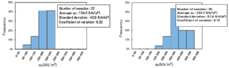
Figure 4. Left, Uniaxial compressive test (ground); right, Uniaxial compressive test (water).
