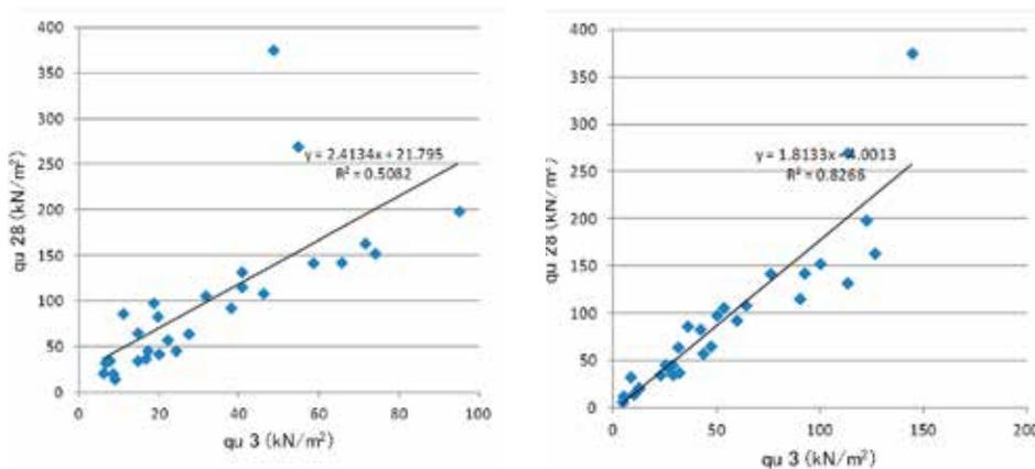
Figure 12. Left, relationship between qu3 soil and qu28; right, relationship between qu7 soil and qu28.
