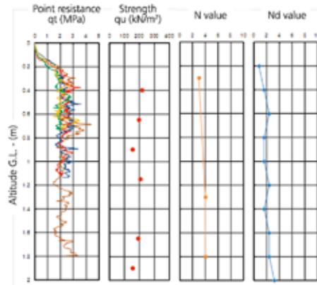
Figure 5. The depth distribution of strength (at age 28 days).
