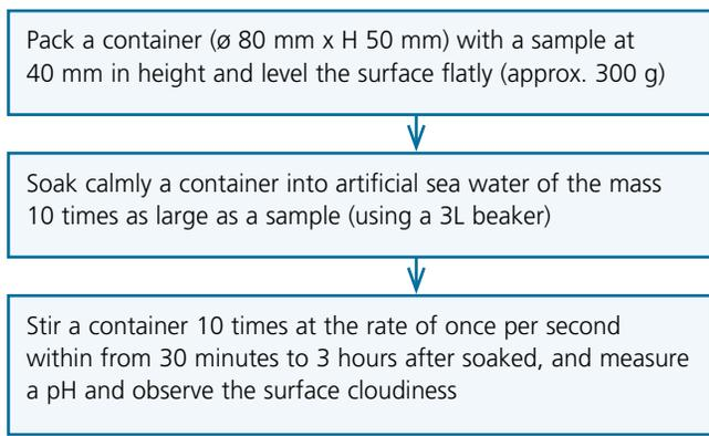
Figure 15. Measurement procedure (Ref 9).
