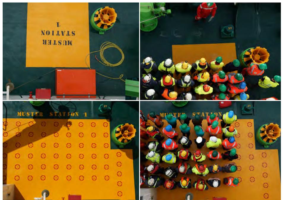
Figure 2: Top left and right: Muster station before painting numbered circles; Bottom left and right: Crew muster efficiently at station with painted numbered circles.
