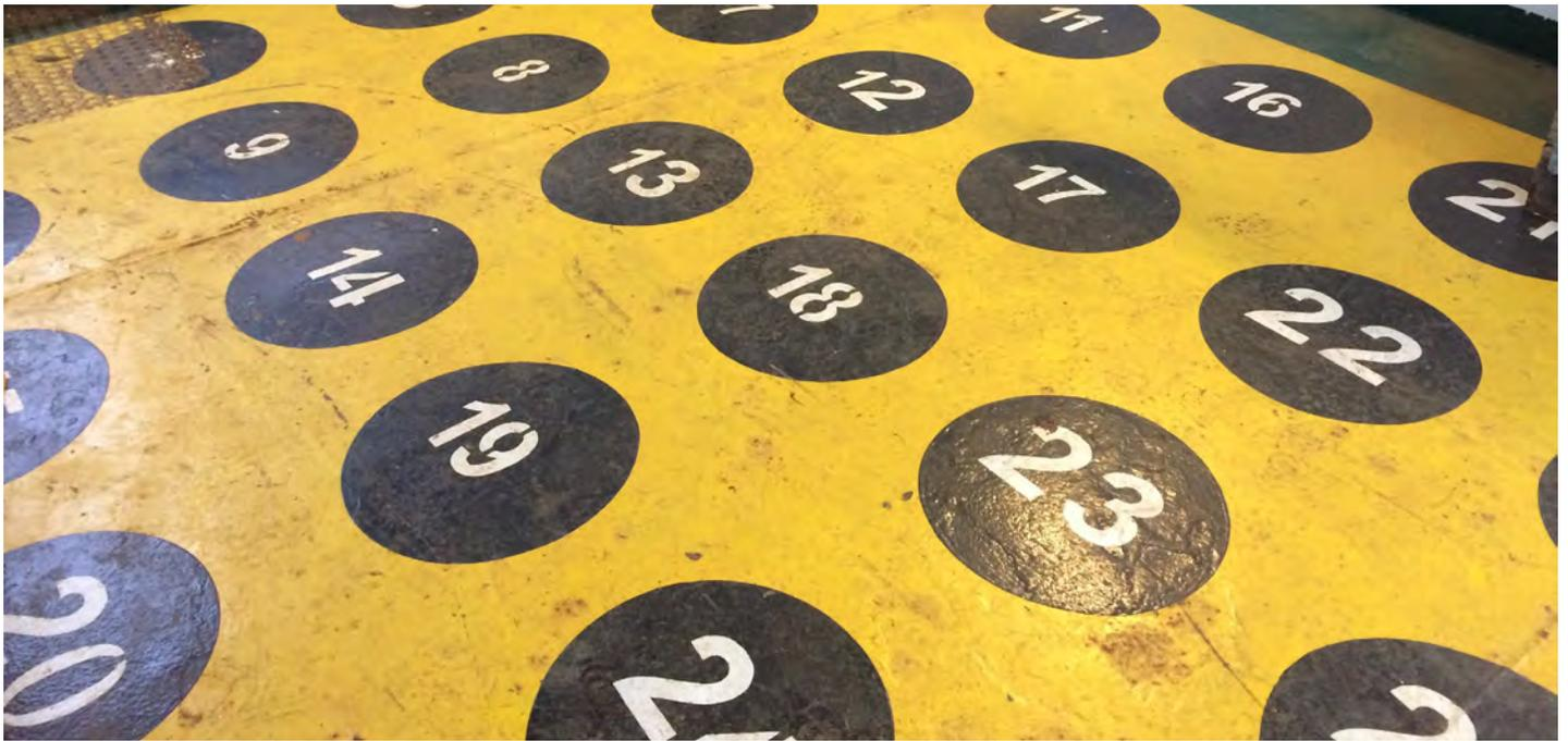
Figure 1: The muster station was enhanced by painting numbered circles on the deck.
