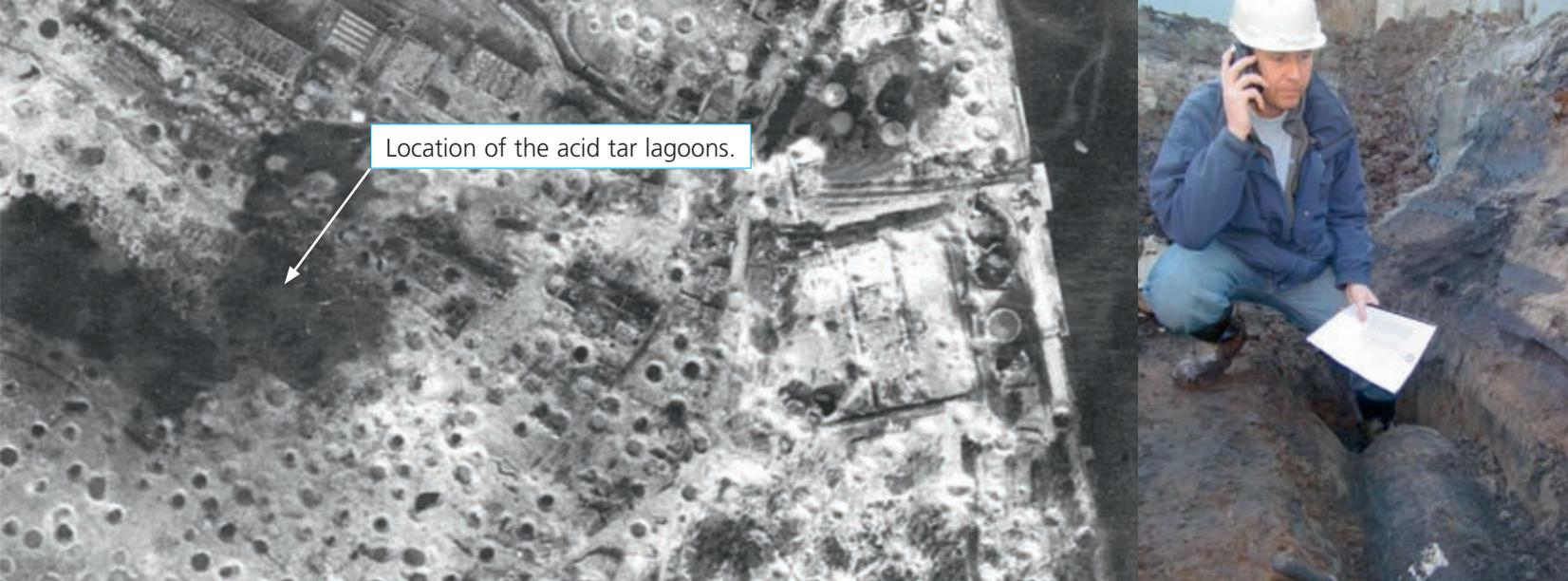
Figure 2. Left, An aerial view of the bombardments of the RAF and USAF in May 1944 and location of the lagoons. Statistically 10 to 20 percent of the total amount of bombs dropped can be expected to have failed to explode.
