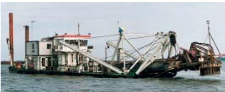
Figure 9. The environmental disc cutter installed on the *Vecht*.
