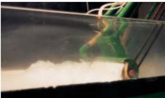
Figure 7. Model test auger, above working without a silt screen and causing turbidity; below, with a silt screen, turbidity is completely absent.
