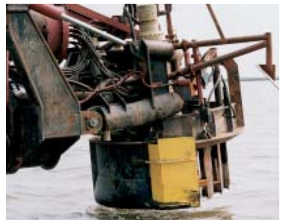
rotating cutter. The mixture is pumped by a centrifugal pump which makes a dilution of the mixture necessary to limit the required pressures for pumping and to limit the decrease in performance of the pump. In order to prevent suction problems the pump is placed directly onto the disc cutter. A control system is required to achieve a high as possible mixture concentration.
