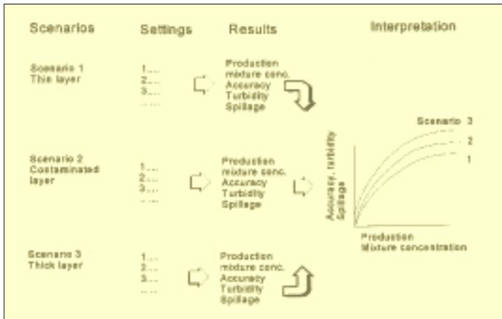
Figure 3. Summary of the method by which each dredging technique is assessed.
