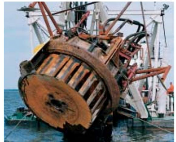
Figure 10. Close up of the environmental disc cutter.
