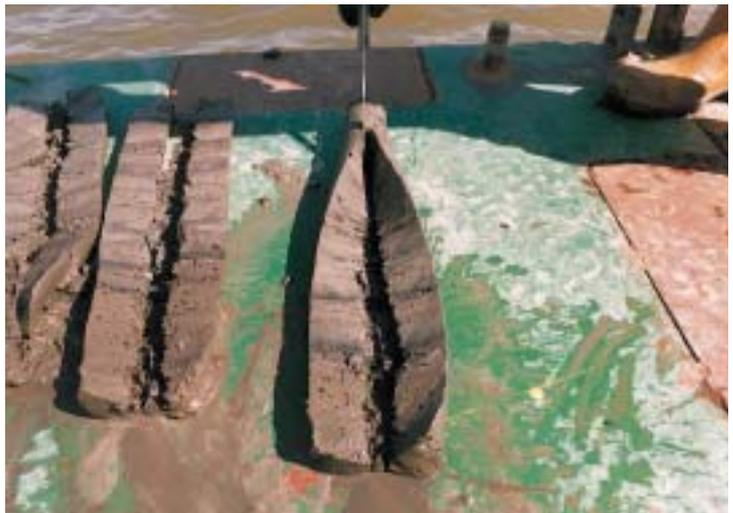
Figure 5. The Beeker sampler (left) with several cut-open samples of a typical core (above).
