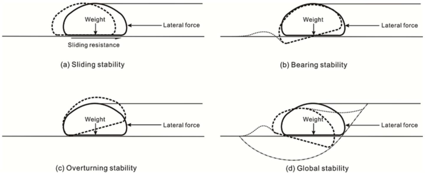
Figure 10. Geotechnical stability checks (adapted from Yee 2002).
