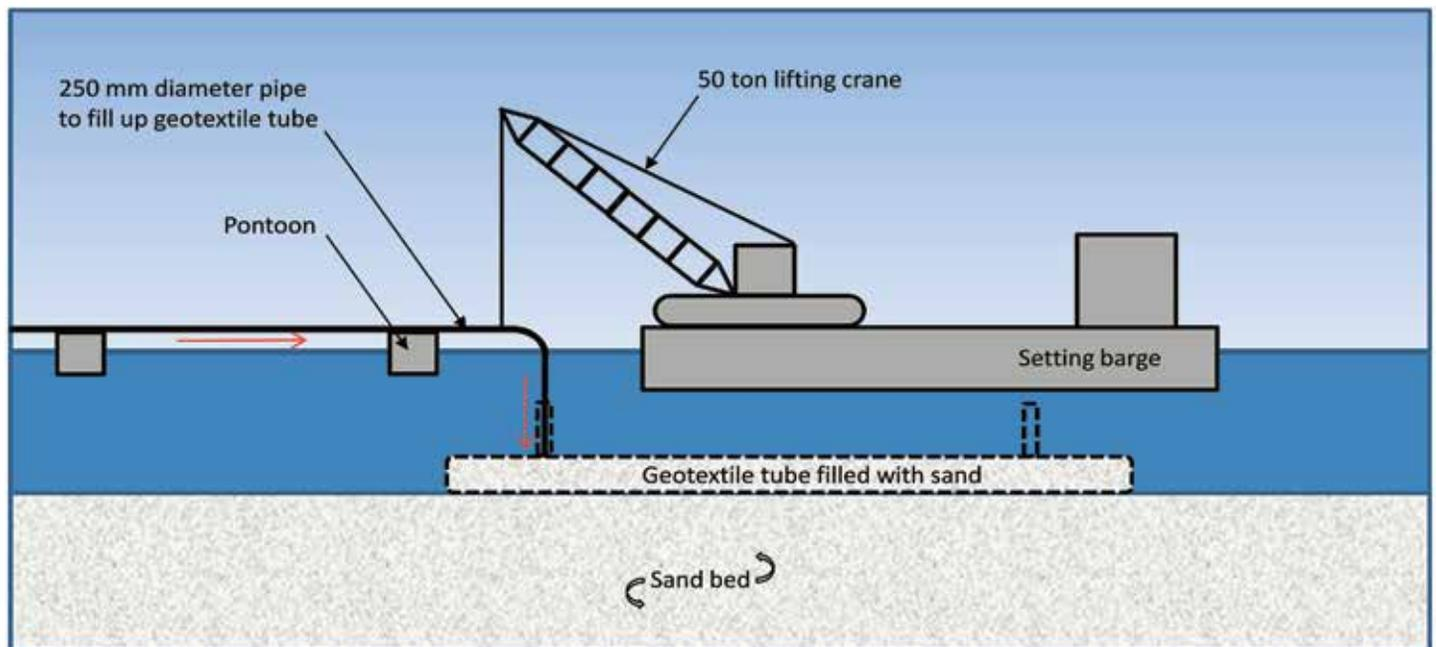
Figure 15. Diagram of the setting barge deployed for the filling of geotextile tube.
