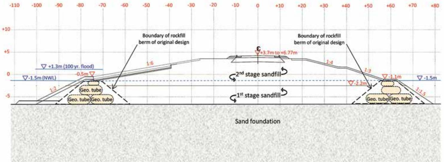
Figure 8. Typical cross-section of the Polder Dike for alternative design with geotextile tube berm (the original design rockfill berm is indicated).
