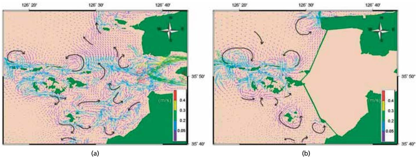
Figure 3. Modelled tidal residual currents of the M2 tides with eddies as potential traps for fine grained sediments (a) before construction of dike, (b) after construction of dike (adapted from Min et al. 2012).
