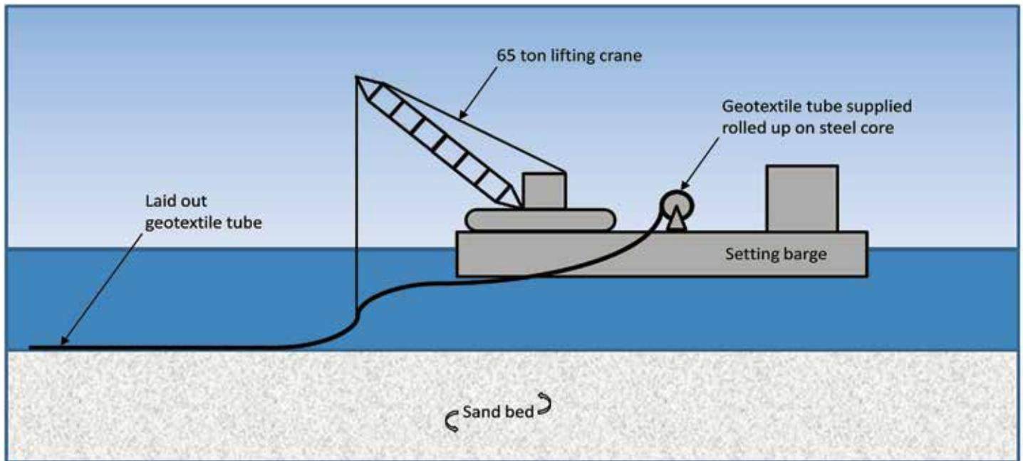
Figure 14. Diagram of the setting barge deployed for laying out the geotextile tube.
