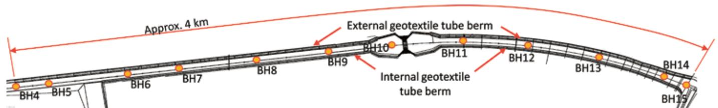
Figure 6. Plan view with geotextile tube berms on both sides of the Polder Dike.
