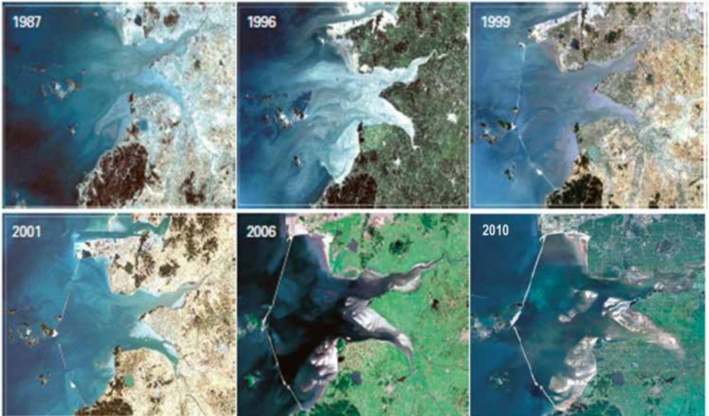
Figure 4. Transformation of Saemangeum estuarine tidal flat into a reservoir from 1987 to 2010 (adapted from Korean Geotechnical Society 2012).
