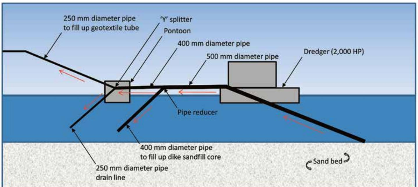
Figure 13. Diagram of the dredger and distribution pipes used to deliver sand for filling geotextile tube and sandfill core of Polder Dike.
