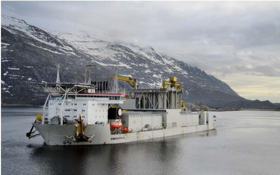
Figure 6. A fallpipe vessel (FVP) being used for subsea rock installation in Norway. Dredging vessels come in a variety of types which may require different fuel solutions.
