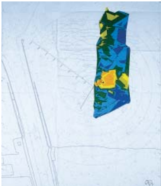
Figure 6. Map indicating the suspended solids in the relocation area 1 metre above the bottom, measured during the works executed with a traditional cutter crown.
