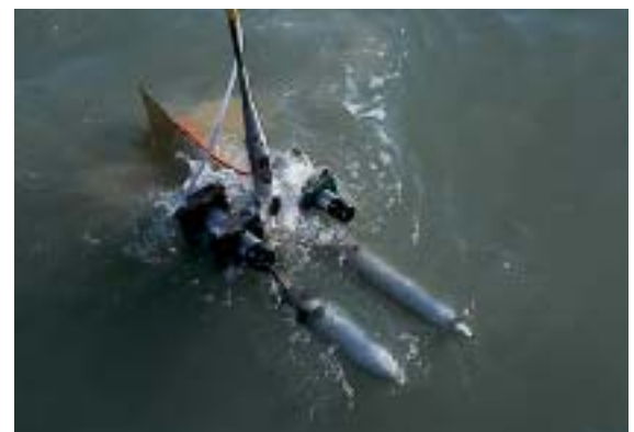
Figure 5. OBS turbidity monitors mounted on the towfish of the Navitracker system for the continuous monitoring of the suspended solids throughout the sediment column.
