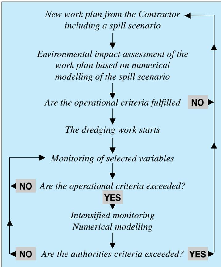
Figure 9. Principals of feedback monitoring.
