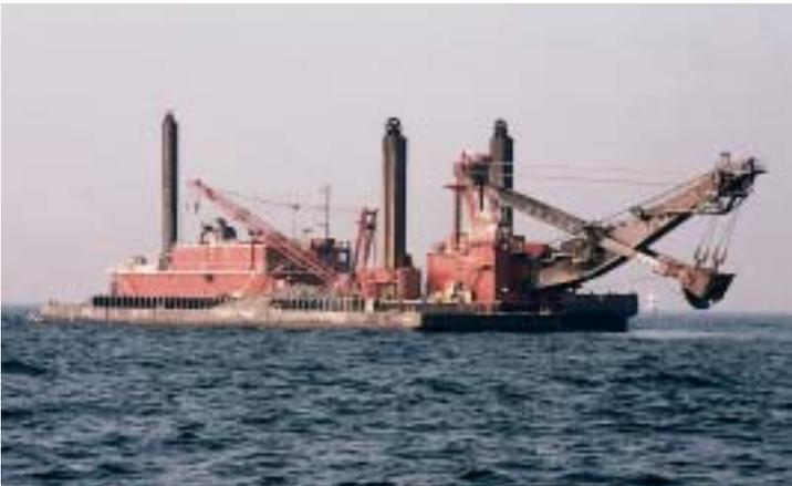
This mechanical dredger works with a bucket which unloads on barges moored alongside the dredger. The filled barges are transported to the landfill areas by tugs, and here the material is unloaded by dozers and mechanical dredgers.
