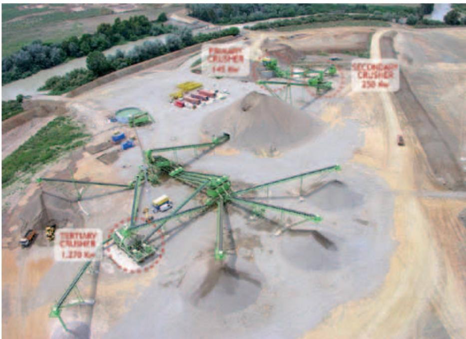
Figure 9. A crushing plant for quarried sand.
