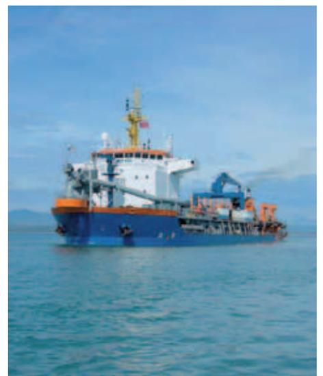
Figure 10. Trailer suction hopper dredger with 10,000 m<sup>3</sup> capacity.
