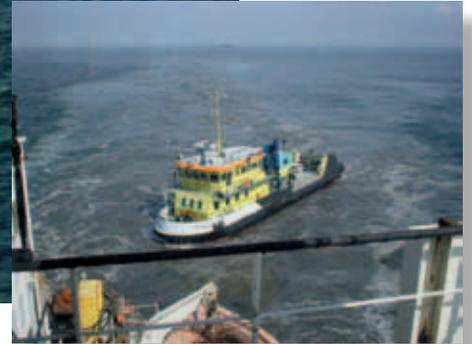
Figure 8. Short, limited extent of plume from a dredger (left), and plume being measured by a survey boat.
