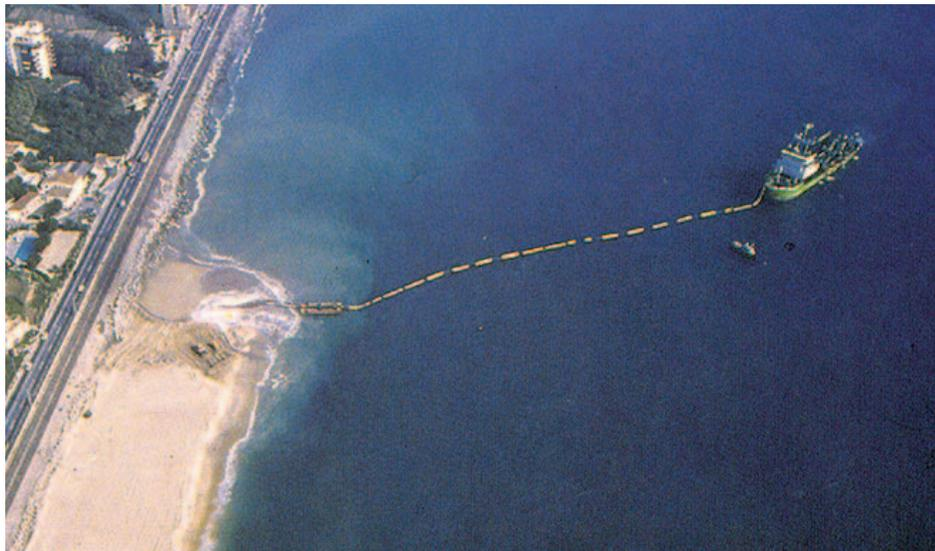
Figure 3. One soft solution is the replenishment of sand, won from a marine bank, by a hopper dredger.
