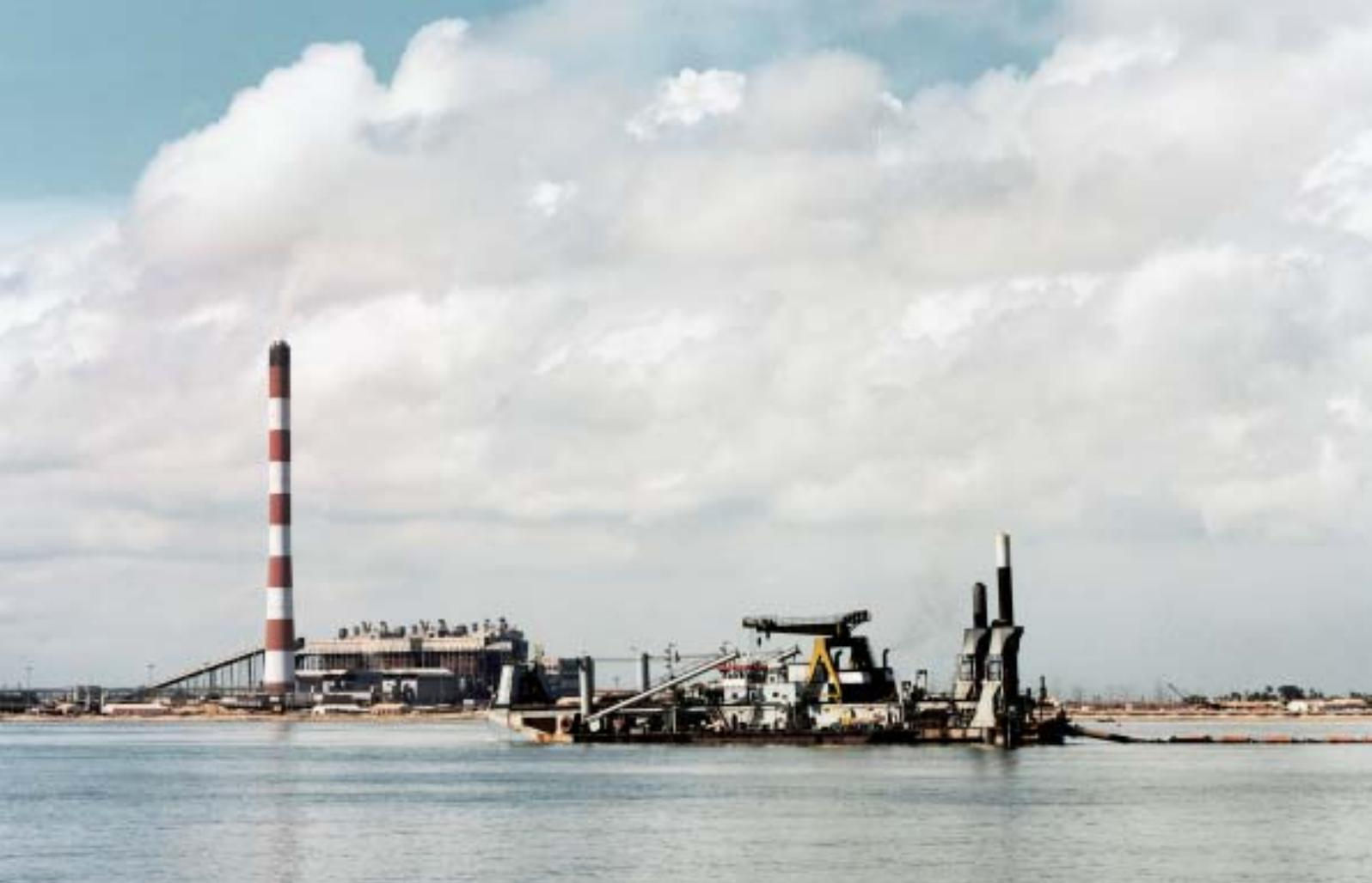
Figure 2. Cutter suction dredger Vesalius, working in front of the North Madras Thermal Power Station.
