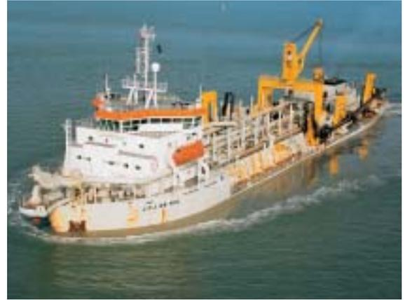
Figure 5. The J.F.J. De Nul, one of the largest trailing suction hopper dredgers in the world, was modified for the new technique of dilution.
