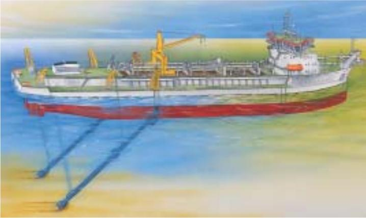
Figure 4. Principles of trench preparation by means of dilution by using a larger trailing hopper dredger.
