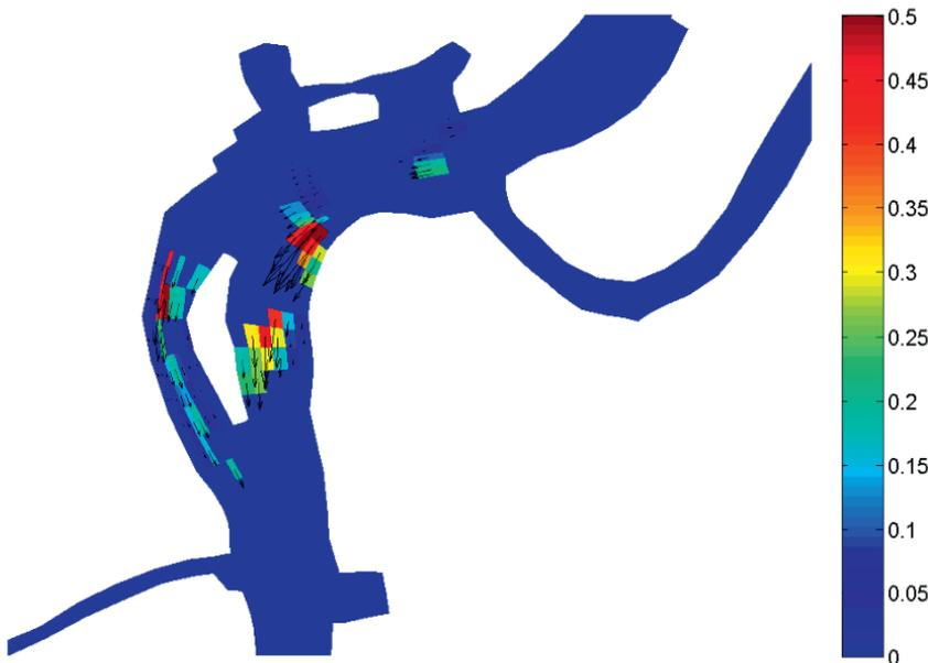
Figure 3. Mean bedload transport rate from January through March, 2012.
