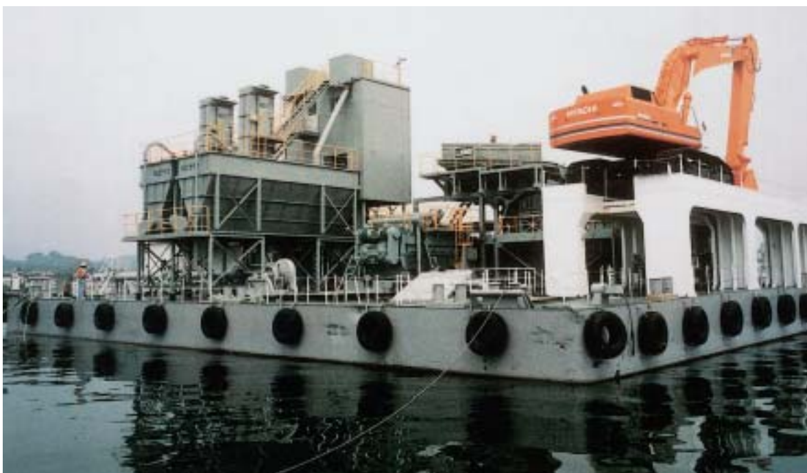
Figure 2. Solidifier mixing plant barge.
