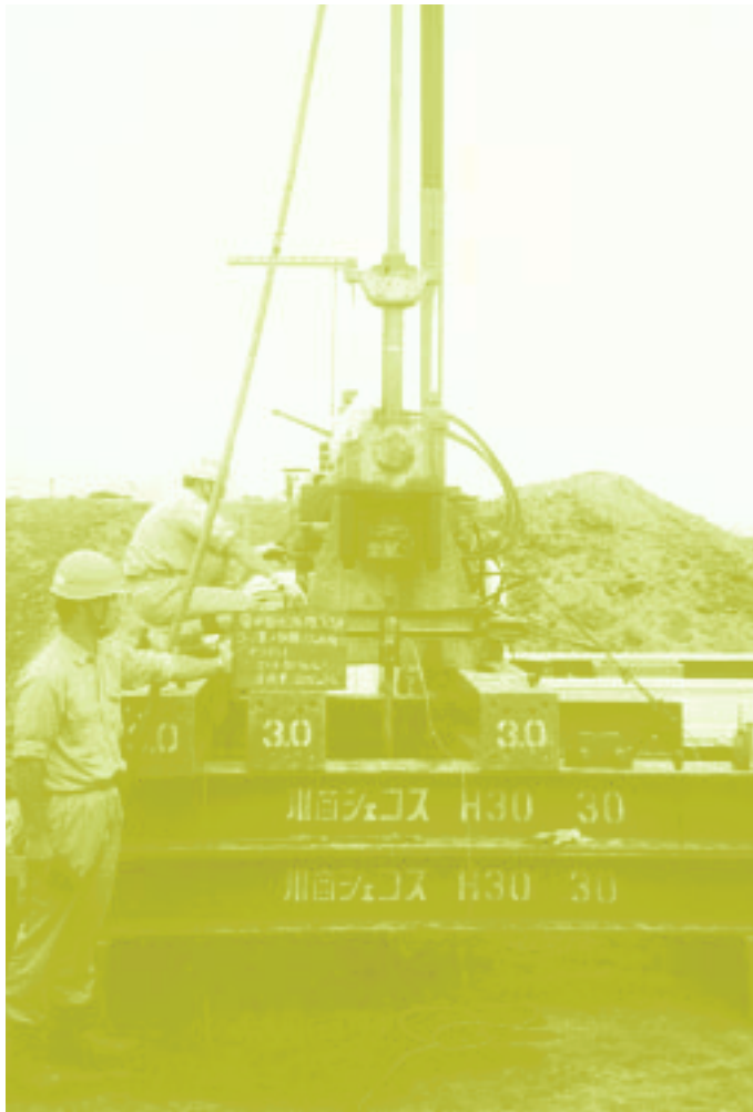
Figure 24. Cone penetration test being performed.
