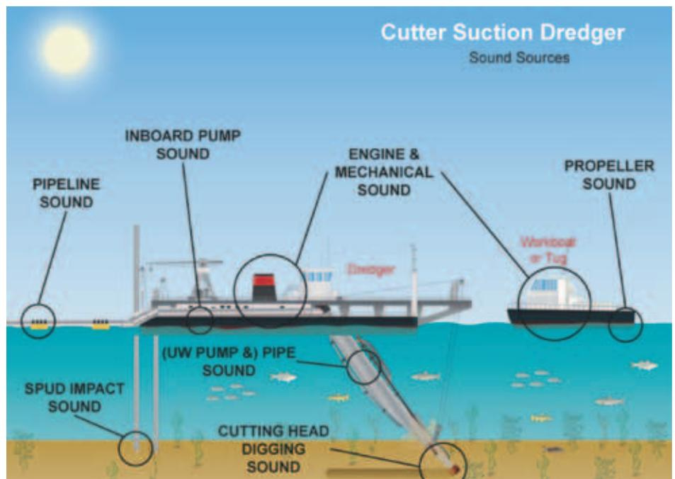
Figure 1. Schematic overview of a cutter suction dredger.
