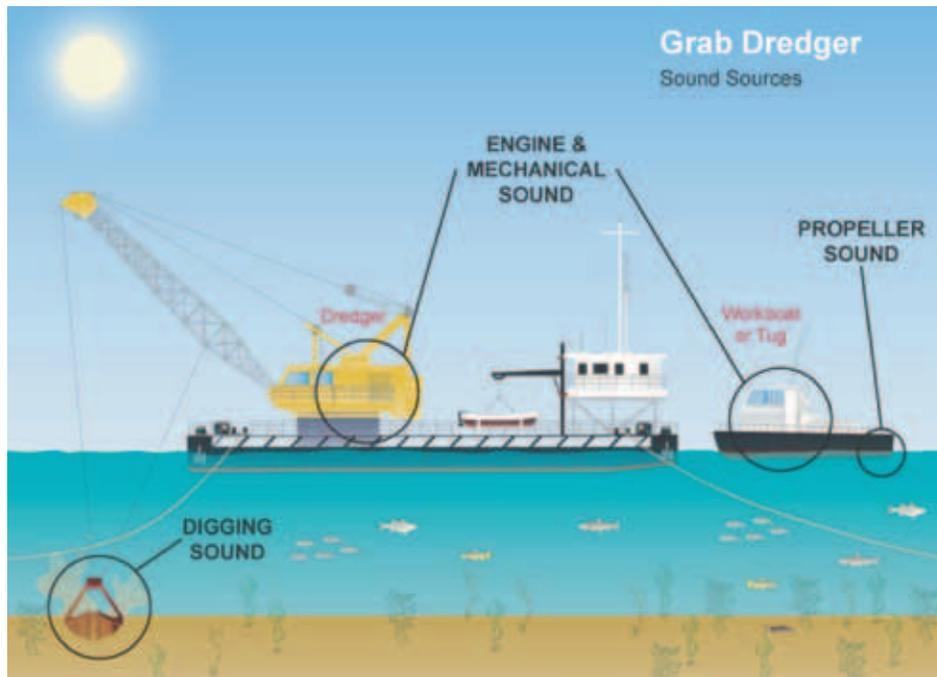
Figure 3. Schematic overview of a grab dredger.
