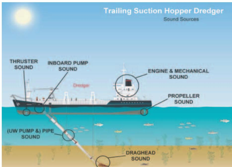
Figure 2. Schematic overview of a trailing suction hopper dredger.
