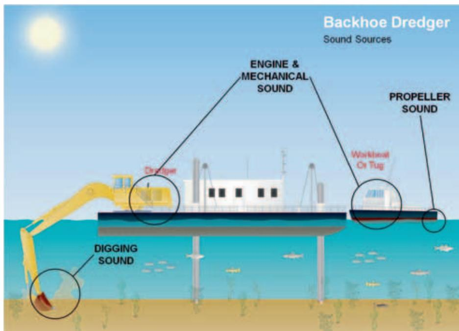
Figure 4. Schematic overview of a backhoe dredger.
