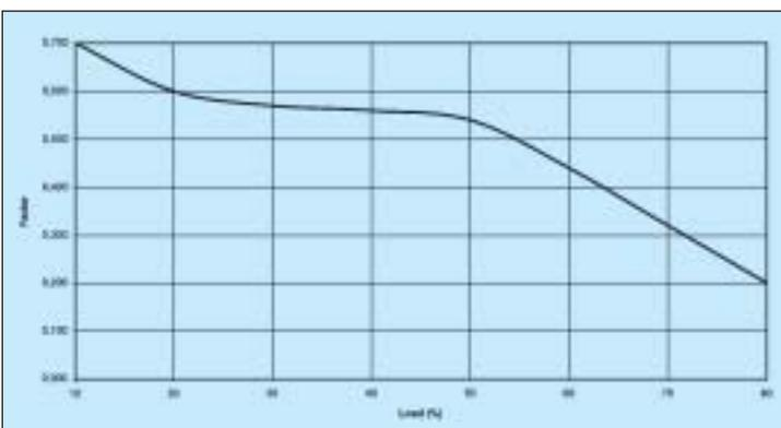
Figure 6. Areal efficiency factor vs. hopper load
