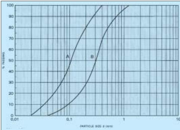
Figure 7. Particle size distribution curve.
