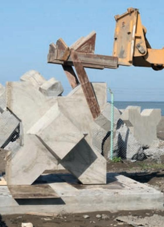
Figure 12. Set-up for the drop tests.
