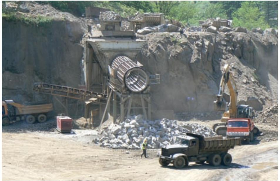
Figure 7. The Drum Screen, the crane and the dump truck.
