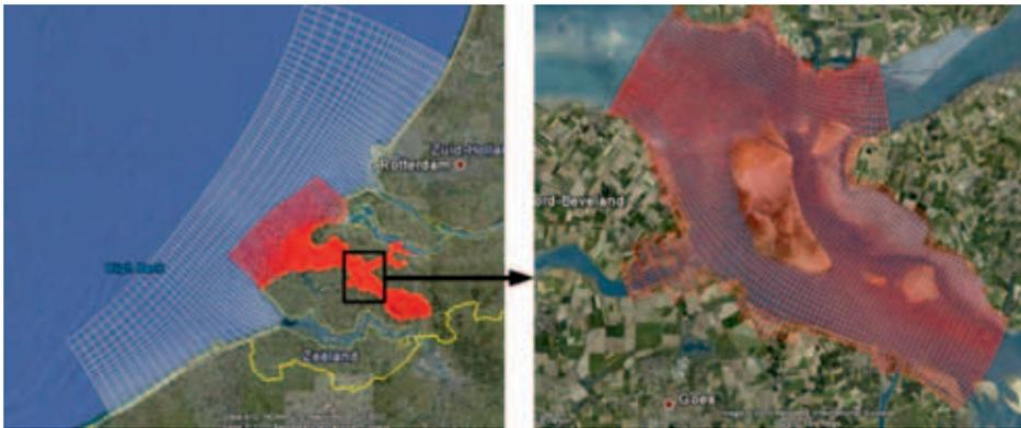
Figure 7. The KustZuid wave grids (left) with the nested Galgeplaat wave grid (right) (Das, 2010).
