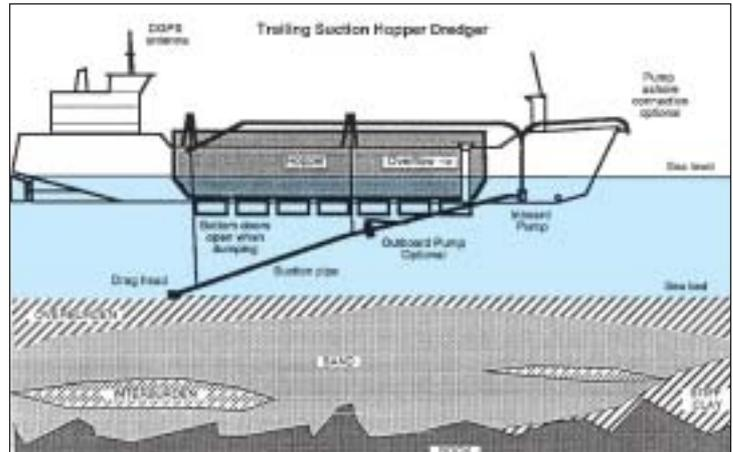
Figure 1. A typical TSHD with a 8000 m<sup>3</sup> hopper capacity is 125 m long x 21 m across with a loaded draft of 9 m. Dredged slurry is discharged in the rear of the hopper. Overflow from the hopper is regulated by adjusting the height of the overflow tubes. TSHDs dredging aggregates have a single dredge pipe, overflow through spillways in the top of the hopper above the waterline, and discharge by pump and bucket wheel or scraper and conveyor.
