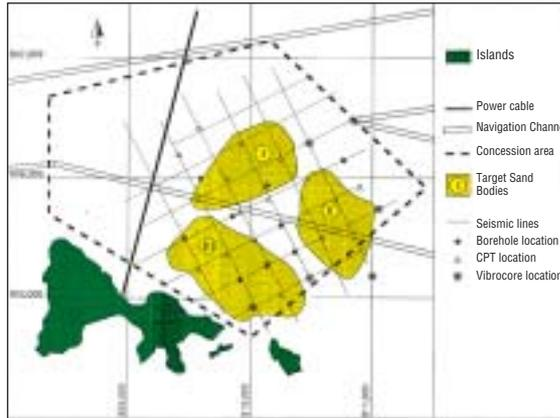
Figure 5. A chart indicating locations of target sand bodies forming potential borrow pits. The example site investigation consists of seismic profiling, sampling and CPTs, however the grid sampling at intersections of seismic lines is not likely to refine the understanding of the sand body. Rather, samples should be placed in geologically representative locations to assess the variability and limits of a resource.
