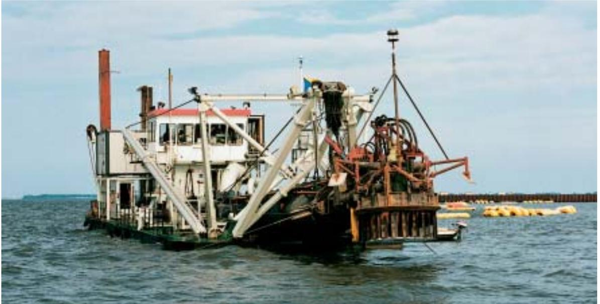
Figure 7. Positioning system of the disc bottom cutter dredger *De Vecht* during dredging trials at Lake Ketelmeer.
