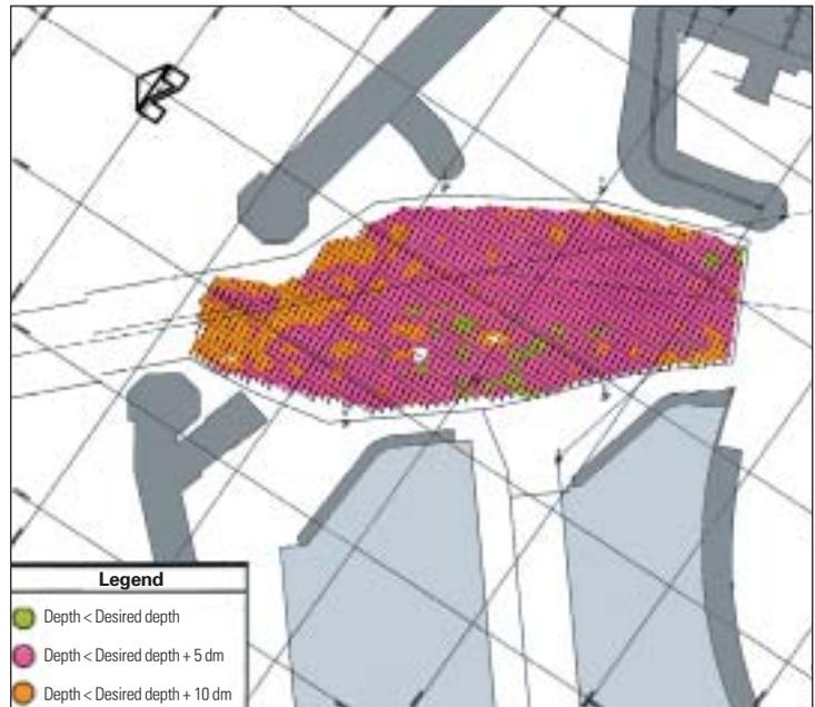
Figure 5. Chart indicating the navigable depth in the Port of Zeebrugge.
