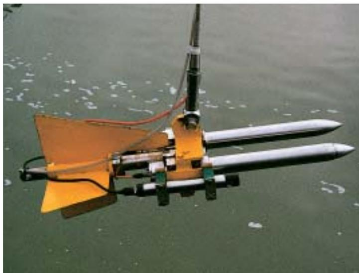
*Figure 8. Optical sensors mounted on the Navitracker VDP, for the environmental monitoring (turbidity, salinity, temperature) of the water column during dredging and relocation operations.*
