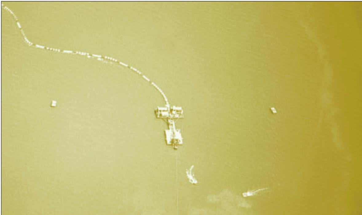
Figure 4. The Willem Bever at work with auger in a box. Specially designed and constructed dredger heads may reduce the turbidity generation substantially. Turbidity clouds seen here in the lower righthand corner are caused by a multicat and the traffic of a working vessel, not by the dredger.
