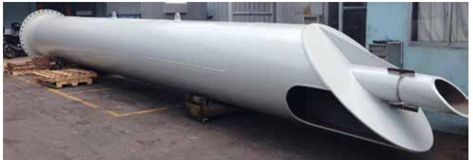
Figure 5. Top photos, installed deep load systems; below, a newly fabricated extended discharge pipe for a TSHD.
