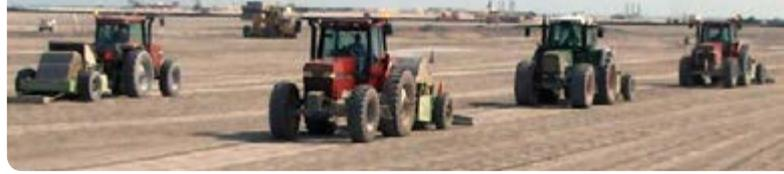
create an impact energy, which provides the compaction. The impact compaction mechanism enables the compaction energy to reach deeper levels than can be reached by normal static bulldozers or vibratory compaction methods.
