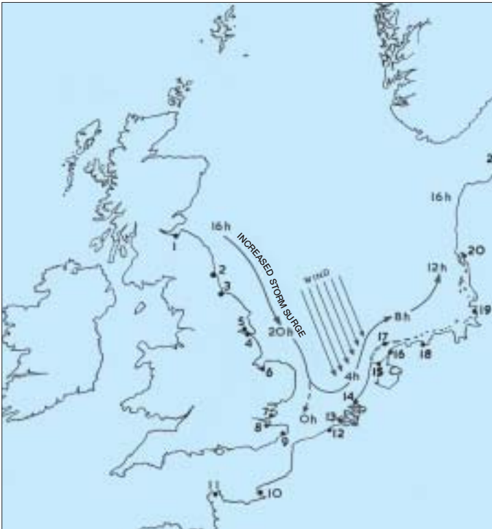
Figure 1. The path of the tidal wave into the southern North Sea with the times of high water (HW) indicated.
