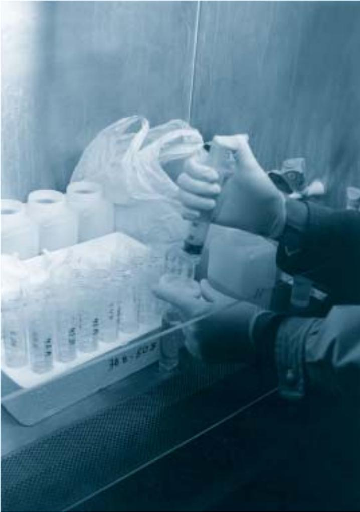
Figure 6. On board the survey vessel, filtration of the seawater samples in a laminar flow workstation were conducted prior to analysis in the laboratory.
