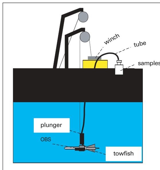
Figure 6. Taking water samples with a plunger.
