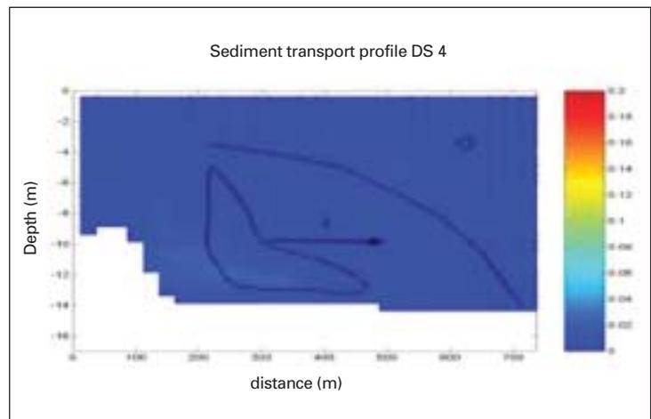
Figure 12. Sediment transport (kg/m<sup>3</sup>/s); neap tide cycle; two hours after low tide; profile DS 4.
