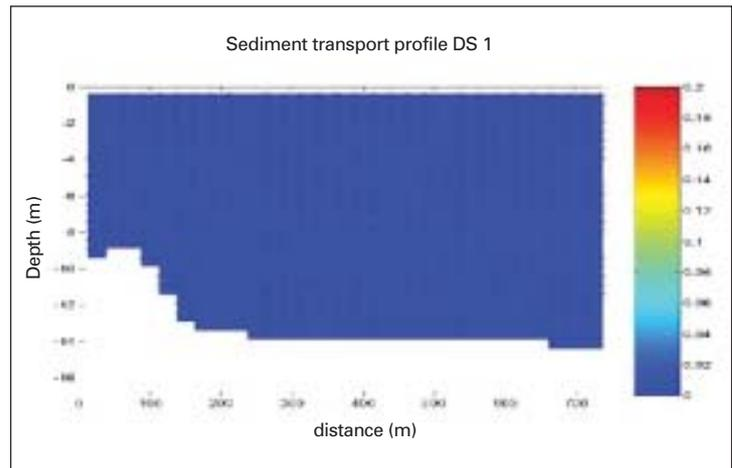
Figure 11. Sediment transport (kg/m<sup>3</sup>/s); neap tide cycle; low tide; profile DS 1.
