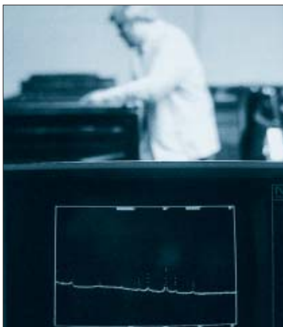
Figure 8. The gamma ray energy spectrum shown on this screen represents several radioactive species being analysed by the germanium-lithium diode detector in the background.
