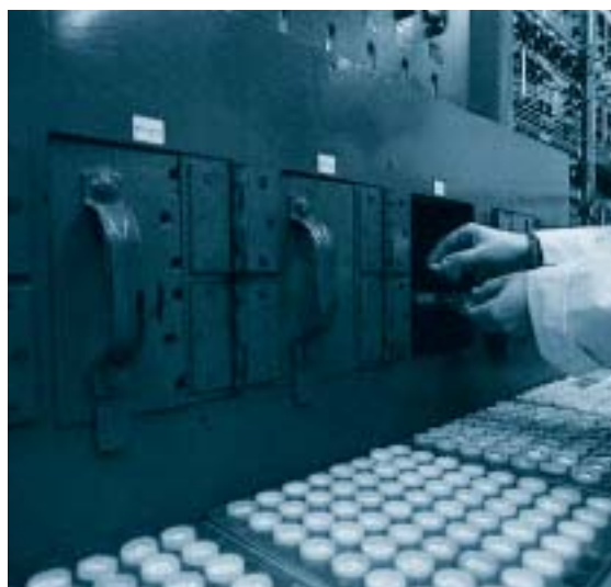
Figure 3. Purified bismuth derived from a sediment sample is loaded into a low level beta-particle detector. The measured radioactivity of Bi-210 is used to calculate the concentration of Pb-210.
