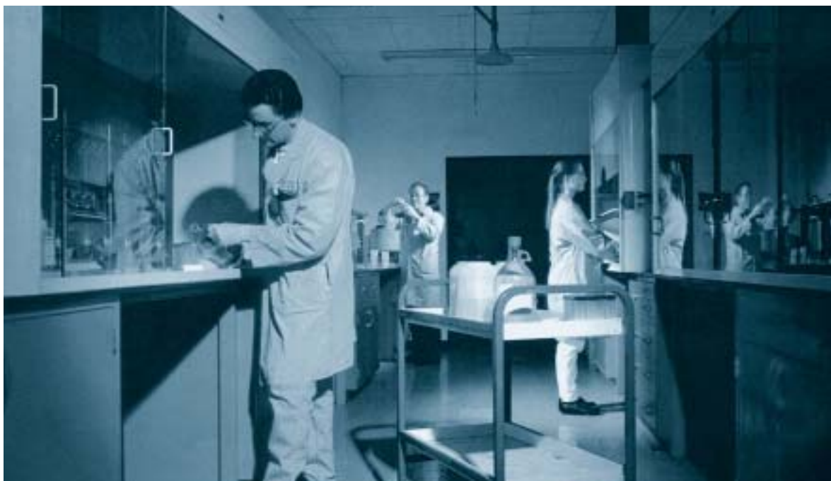
Figure 2. Radiochemical separations are performed to isolate bismuth or polonium from sediment samples. The purified elements are then analysed in radioactivity detectors.
