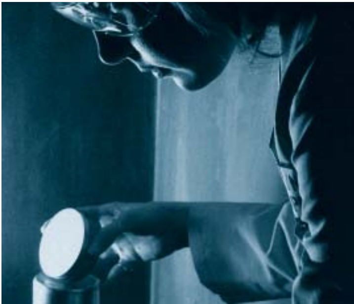
Figure 7. A sample prepared in a standard cylindrical container is placed on a germanium-lithium diode detector to measure its gamma radiation.
