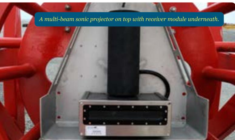
*A multi-beam sonic projector on top with receiver module underneath.*
