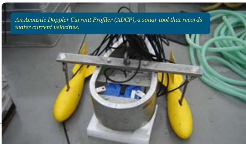
*An Acoustic Doppler Current Profiler (ADCP), a sonar tool that records water current velocities.*
