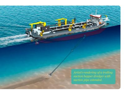
into the hopper. There the solids settle out and are held awaiting transport and subsequent placement.
