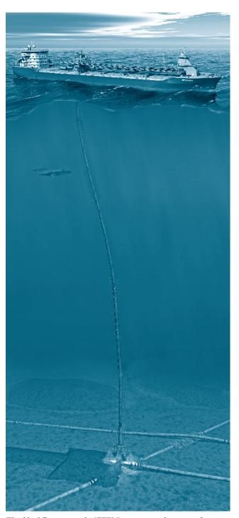
Flexible fall pipe vessels (FFPV) are primarily operated in very deep water up to 2,200 metres, when covering oil and gas pipelines, levelling the seabed or applying scour protection. An ROV is attached at the lower end of the fall pipe for better positioning.
