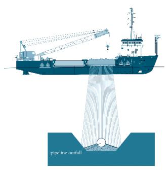
Side stone dumping vessels (SSDVs) are self-propelled ships that are typically used to install scour protection for offshore wind turbines and offshore rigs, to construct breakwaters or to install rock for subsea pipeline protection.
