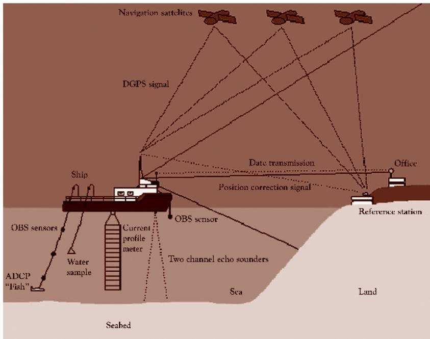
This schematic drawing shows an environmental monitoring vessel and the wide variety of survey equipment available, such as echo sounders, a current profile meter, OBS sensors and DGPS navigation satellites.
