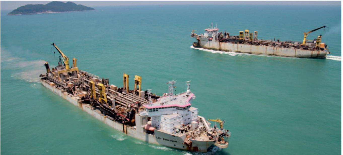
The two sister THSDs *Cristóbal Colón* and *Leiv Eiriksson* both have a hopper capacity of 46,000 m<sup>3</sup> and a maximum dredging depth of 155 m
