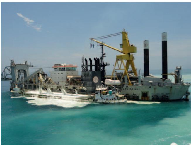
*CSD J.F.J. De Nul is the world's largest cutter; with a total installed power of 27,240 kW, she can dredge to 36 m depth*
