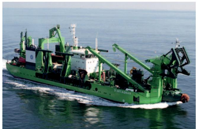
*The self-propelled heavy-duty CSD D'Artagnan has over 28,000 kW total installed power and can dredge from 6 to 35 metres depth*
