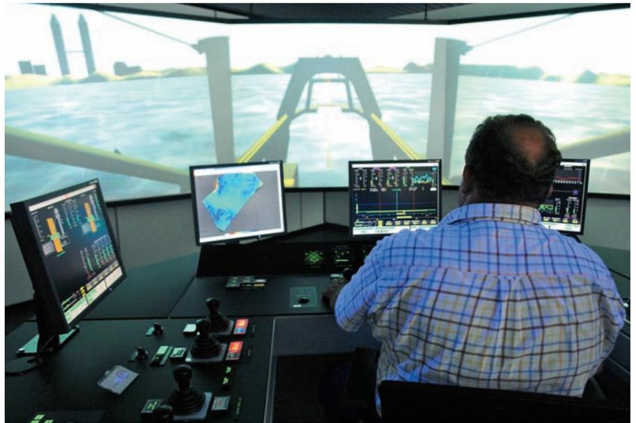
An example of the kind of high-tech training being used for dredging personnel: A training simulator for a cutter suction dredger.
