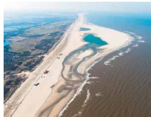
An aerial view of the Sand Motor (also known as the Sand Engine), an artificial peninsula on the coast near Ter Heijde/Kijkduin in the Netherlands. It is an innovative pilot project developed to nourish the coast naturally. The Sand Engine is one of the projects analysed using the ES concept.
