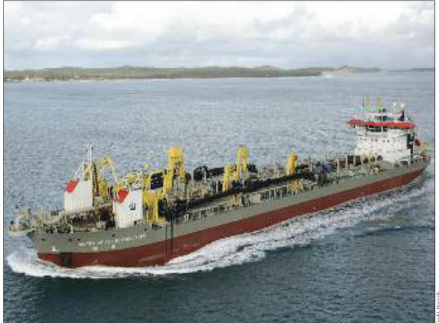
**FIRST PLACE:** Melbourne trail-blazed with the world’s first cutter fitted to a trailing suction dredger
